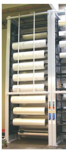
For straight-edge guiding the paternosters can be moved on rails. Control is via an electric light barrier.
