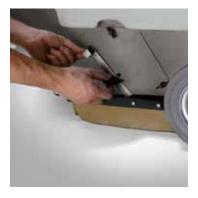
The central broom height can be easily adjusted without any tools
