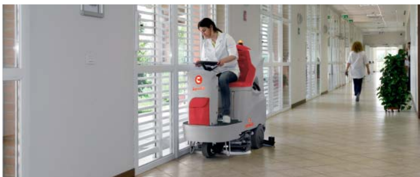
The suction head is silenced, guaranteeing a very low acoustic pressure level and allowing to perform in highly noise-sensitive environments such as nursing homes and hospitals, without disturbing the environment or the people who live in it
