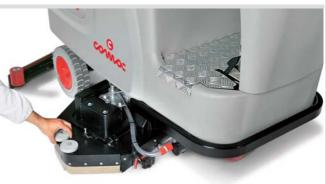
The sweeping-scrubbing unit has been designed to offer a solution to more demandino cleaning tasks and it is suitable for more stubborn dirt. It is in fact provided with a cylindrical brush system which, not only scrubs, but also picks up solid dirt (cigarette butts, wood shavings, small metal residues, etc.) and conveys it into a special hopper which can be easily removed for emptying
