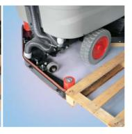
When the squeegee and the scrubbing head bump against an obstacle, they just follow its contours and automatically go back to their normal position as soon as the obstacle is out of the way. This mechanism is extremely important to clean in complete safety along walls and shelving
