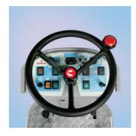
All the main controls are positioned on the dashboard so that they are conveniently accessible and easy to read from the driver's seat
