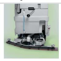
Thanks to a little hose in the rear part of the machine, the level of water in the solution tank is always under control.
