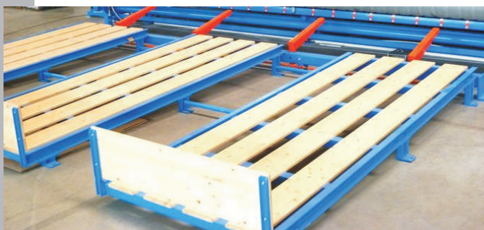
Return path, leads the rolls away from the supply table and cutting machine
