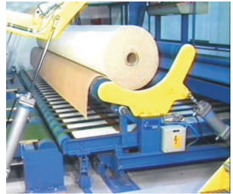
Compensator with edge control, to unpack, handle, back-wrap, pile outside or inside
