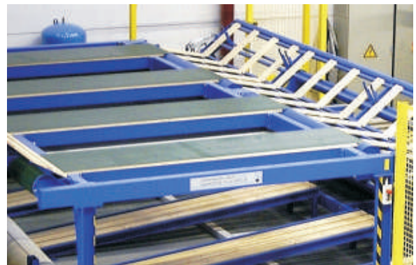
Supply table to store and buffer the rolls for continuous work with the cutting machines
